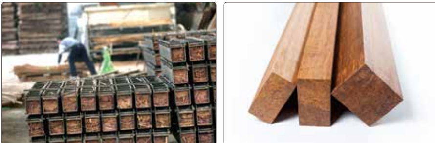
Figure 10: Strand Woven Bamboo beams are made by compressing rough bamboo fibres in moulds under very high pressure (photos MOSO International)
